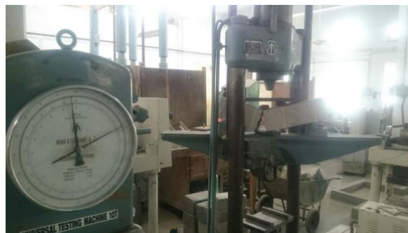
Fig. 3 Testing of specimen for flexural strength
